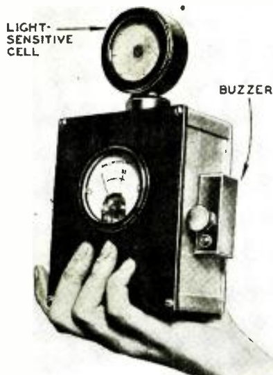
Fig. B The photoelectric guide unit, with its photronic cell on the top and a buzzer on the side.
